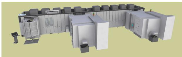
Mach Machine, Inc. recently expanded its automated production capabilities with the addition of two Okuma MB5000H attached to a 24-station Flexible Manufacturing System (FMS). This is a lights-out manufacturing system that operates unattended, day and night.
